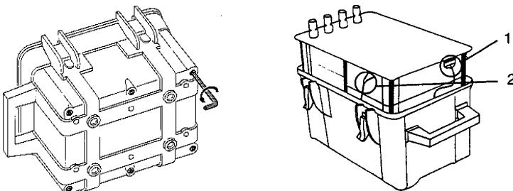
Lift away the chassis without forgetting to disconnect the linking cables 1 and 2 connecting the power supply board located at the bottom of the case to the upper board fixed on the chassis.
