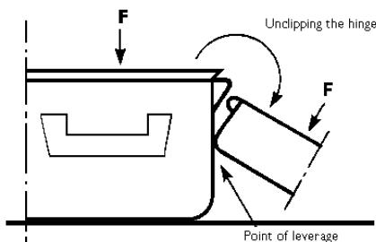
To refit the lid, locate the hinges in their recesses and press hard from the back to the front of the lid until it clicks into place.
