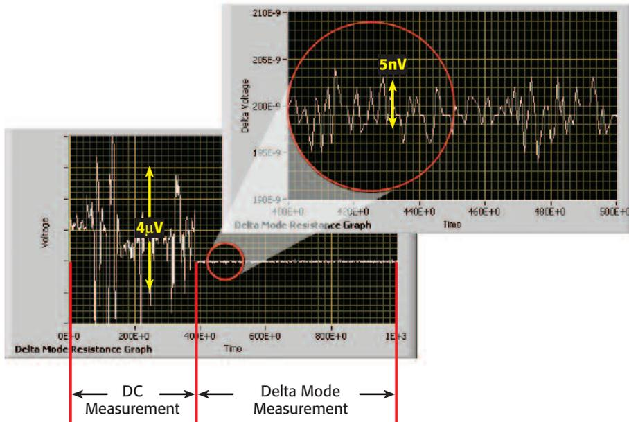
Figure 2. Delta mode offers 1000-to-1 noise reduction.
