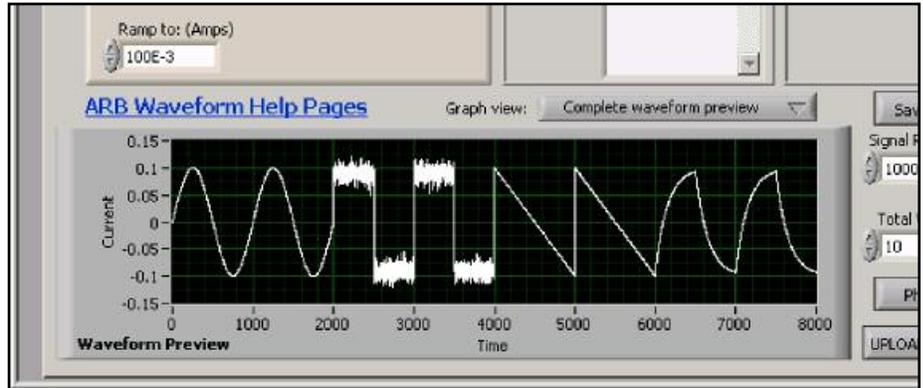
**Figure 4.** The Model 6221 and the free start-up control software supplied make it easy to create complex waveforms by adding, multiplying, stringing together, or applying filters to standard wave shapes.
