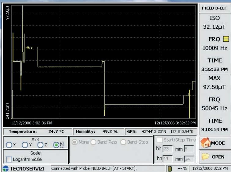
▲ **ACQUIRE** Mode: current ELF measurement graphic displaying instantaneous value (ISO) and maximum value (MAX).
