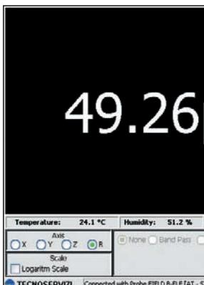
**ACQUIRE** Mode: current RF measurement graphic displaying instantaneous value (ISO), maximum value (MAX) and mobile median value on a six-minute interval (AVG).
